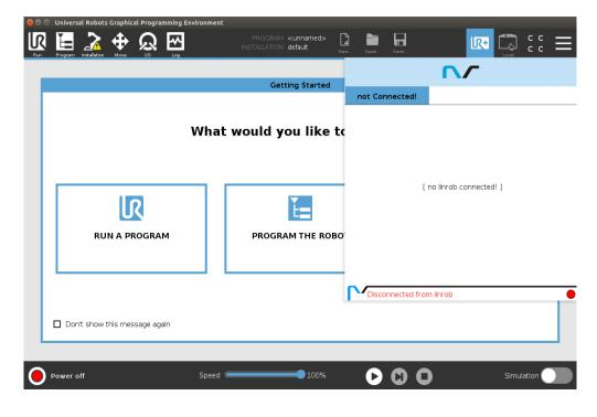
Therefore, tap the *Installation* button at the top of the left side. Then, tap the *URCaps* button in the navigation panel on the left side. Select *"linrob Setup"* in the dropdown list.
