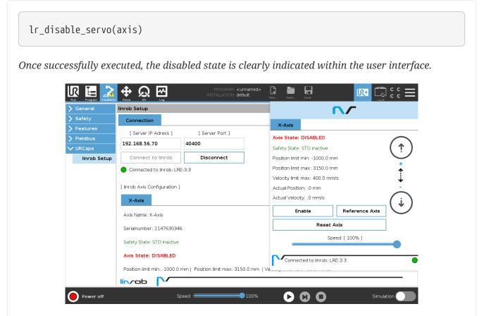
This function disables the drive and applies the break, if available. The attached axes are not operational and in a safe state.
