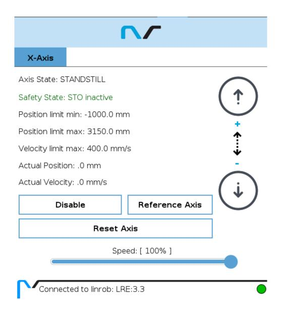
The "UR+" toolbar, displayed in the top right corner, is a quick access toolbar, provides jog controls, an enable/disable toggle, referencing and reset, and displays current axis data for efficient operation.
